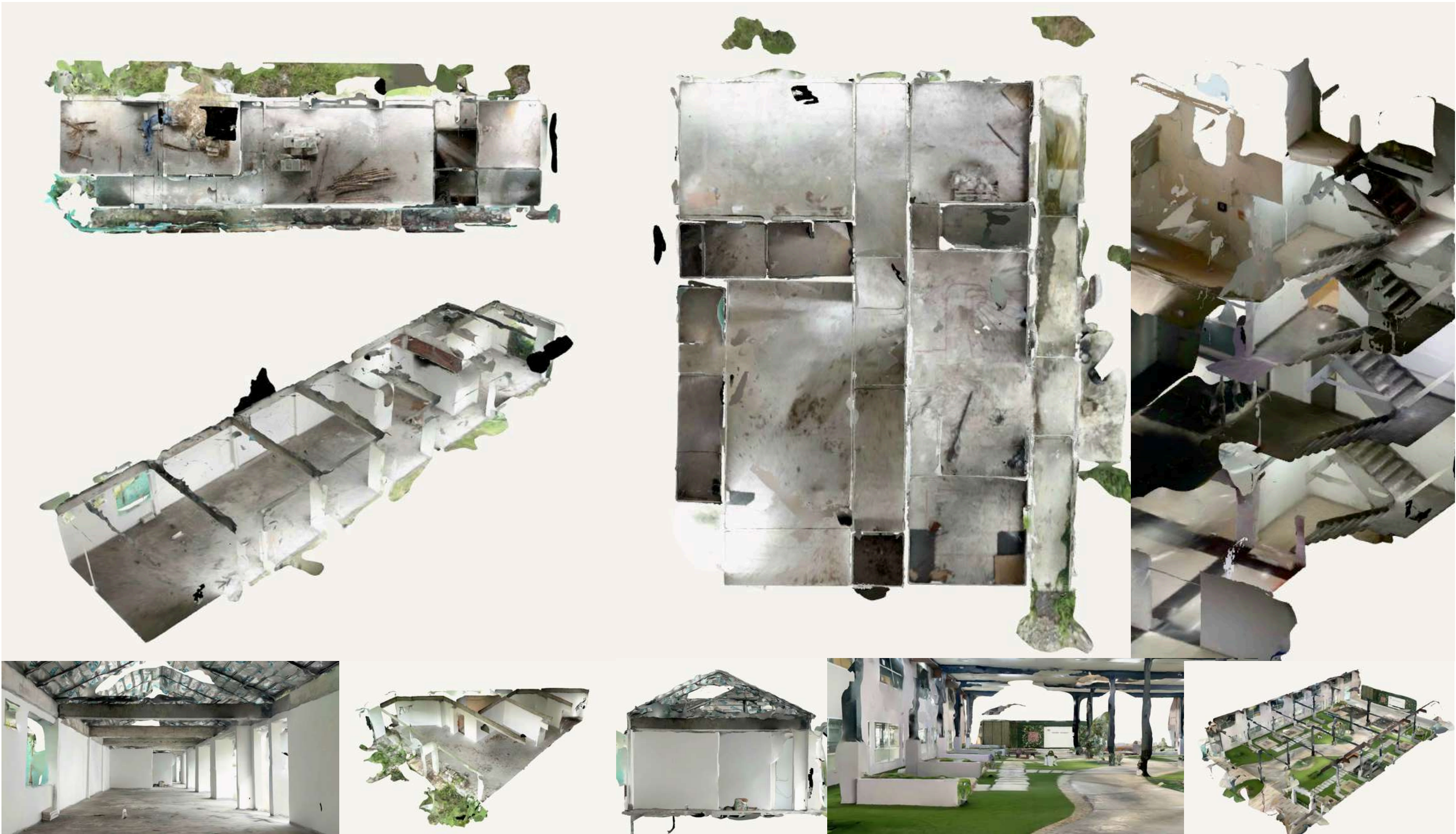
Site Survey & Existing Condition Documentation Conducted an on-site survey for the renovation project, using Polycam on a mobile device to perform 3D scanning and capture accurate existing dimensions, spatial conditions, and architectural elements for further design development.
